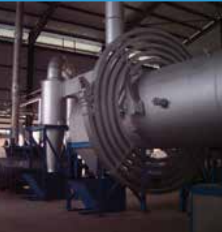
High temperature rotary kilns are used to remove contaminates from spent activated carbon.
