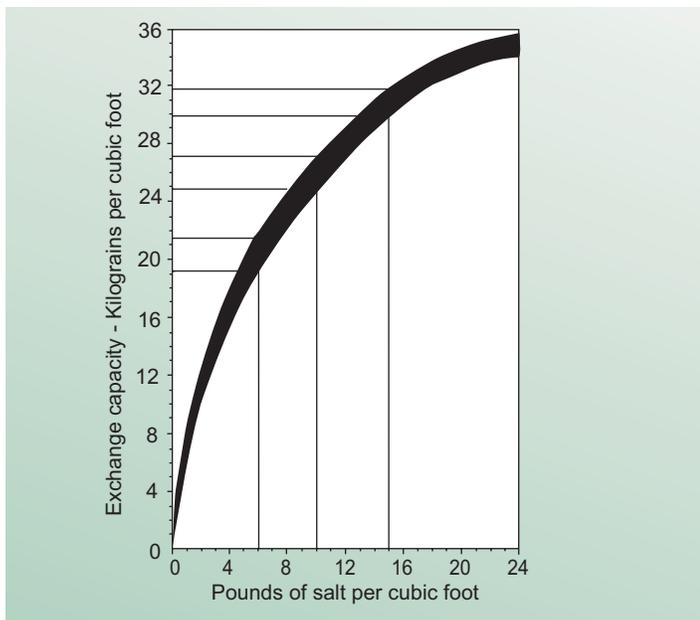
Fig. 1 Exchange capacity vs. regeneration level Sodium form C-700 Cation Resin
