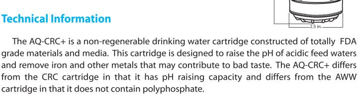
The AQ-CRC+ can be used alone or as a pre-treatment for other cartridges such as a carbon block. It is ideal as a polisher for drinking waters that have been stored in metal tanks or as a pre-treatment for R/O.
