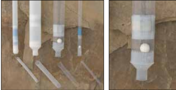
Polyethylene bailers are opaque; PVC and FEP bailers are clear.
