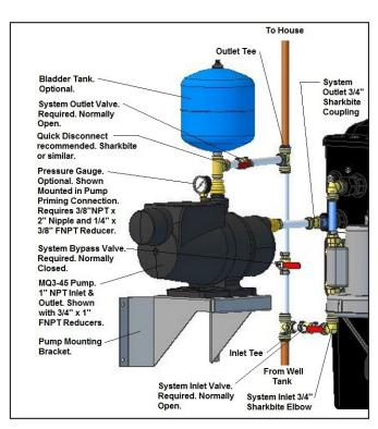
**Figure 2**Pump & Bypass Assembly
