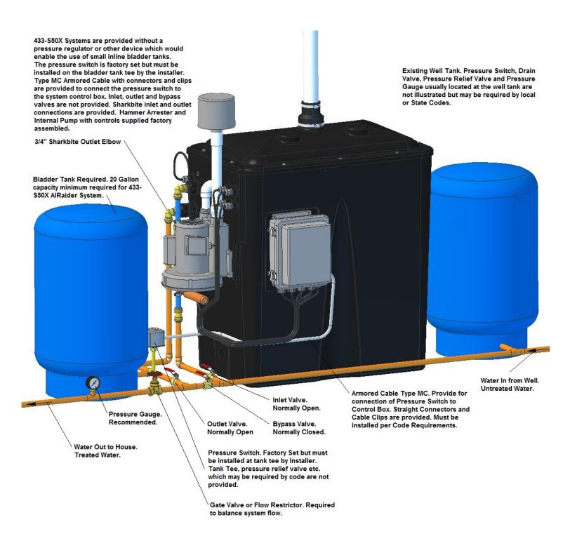
**Figure 5** Plumbing Installation 433-S50X
