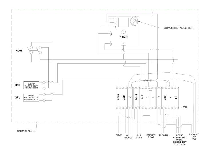
**Figure 6**AIRaider 321ND and 433ND Wiring Diagram 115V
