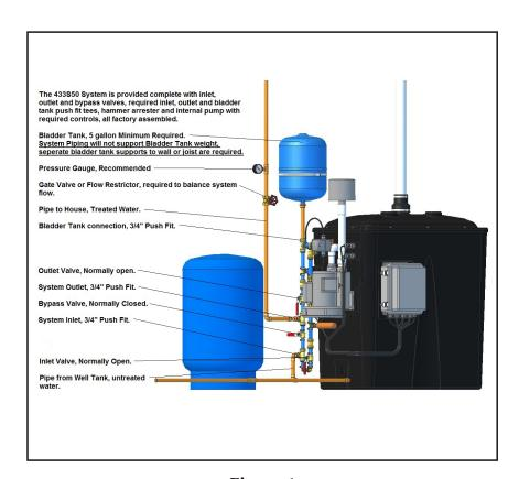
**Figure 4**Plumbing Installation 433S ND System
