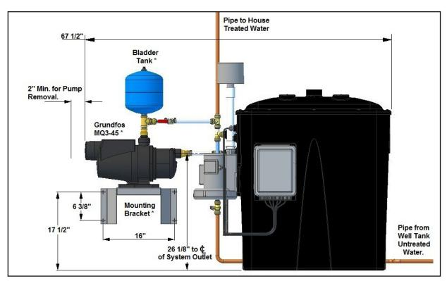
**Figure 3**Installed 433 ND System
