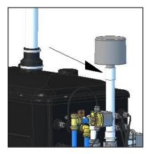
**Figure 12**Air Intake Connection
