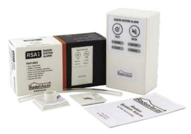
RadonAway's new vacuum monitoring alarm utilizes piezoresistive pressure sensor (PPS) technology and provides audible and visual indications when the radon system is not moving sufficient air to be effective. It is designed for use on 2", 3", 4" or 6" pipe, or flat surfaces. Some of the RSA1's additional features are:
